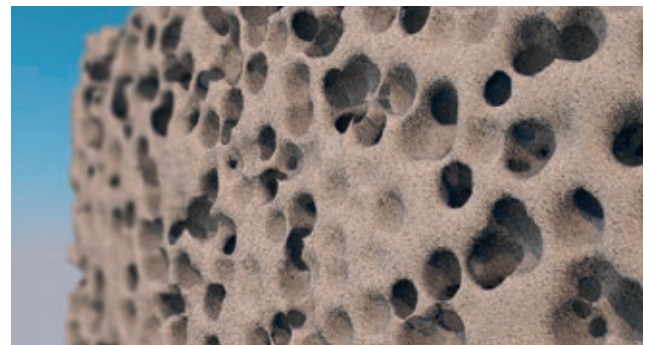
The interlinked macropores facilitate the transport of moisture and the salts dissolved therein to the component surface.
