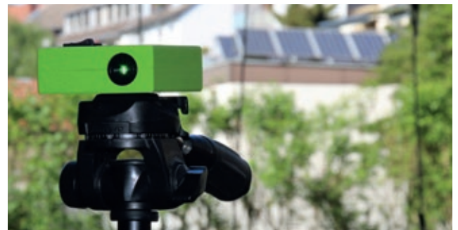
The injection process is permanently monitored using laser-based soil and structure control equipment.
